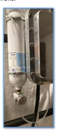
To create a leak free connection when attaching the demand regulator, it is suggested that a small amount of petroleum jelly is added to the threads and O-ring of the regulator.
