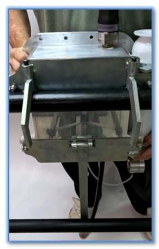
The Rigwire System has an integrated hand rail mounting system attached to the back of the case. This mounting hardware folds up easily for transport of the equipment and folds out quickly and allows the user to mount the Rigwire System on a common hand rail in seconds.
