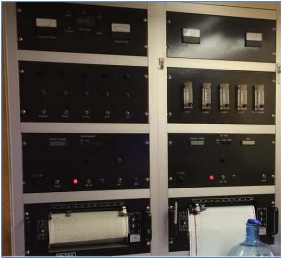
As the electronic age emerged and the systems became more advanced, reliable, and precise, the simple deflection on the face of a meter was not acceptable for long-term logging while drilling a well. As the 70's and 80's came of age, more digital equipment found its way into the logging arena. As such, the semi-digital equipment was not able to compute or display decimal points or parts of a percentage.
