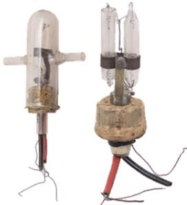
As this sensor technology was perfected over time, and evolved into more reliable and better equipment, many thousands of instruments were built and used for many years using Platinum and then also Nichrome wire filaments.
