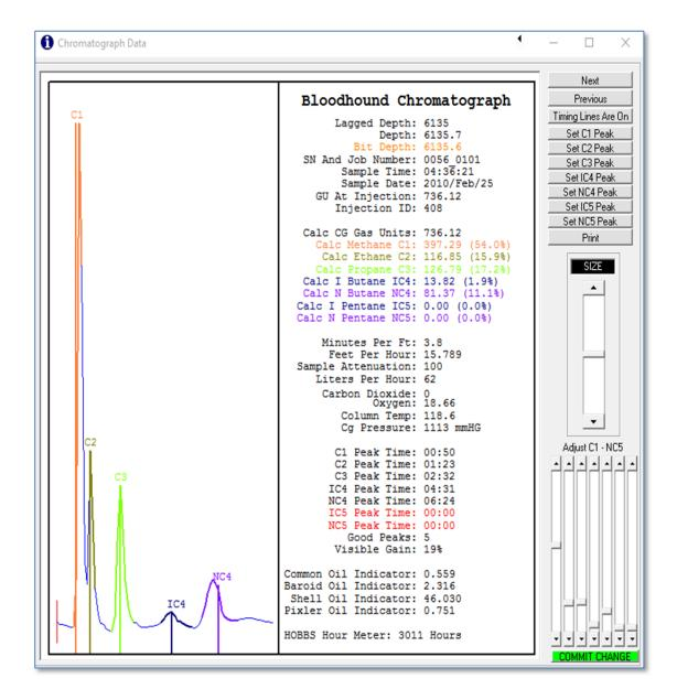
This button allows the user to see a close-up view of the selected chromatograph output. Left clicking and holding on the chromatogram will allow the user to adjust the trace up and down on the display window. If the trace is too large or too small, the user can adjust the over all visual size in the Program and Equipment Setup Screen, under the Chromatograph Tab. When the user is satisfied with the display, a print can be made of the chromatogram.
