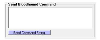
When using this CLI interface you will need to have the Bloodhound tab open in Setup as well as the Real Time Data window in order to send and view commands. When you type the command in this window you need to click the Send Command String after each command and view the results in the RTD
