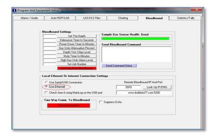
In the Edit box to the right of the Use Ethernet radio option you just selected, you need to type in the LAN IP Address and Port you collected in Step # 2 above. Delete the DNS Name and Port currently in that Edit Box (i.e. <a href="https://www.iballdata77.com:5300">www.iballdata77.com:5300</a>) and then type in your LAN IP/Port.
