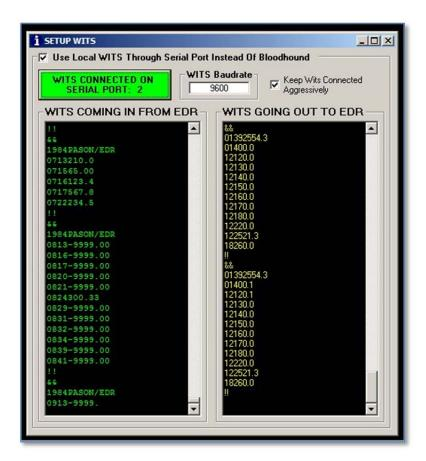
Normally the Bloodhound will be connected to the WITS source of data and Gas Chart will accept the data directly from the connection to the Bloodhound only. If the Bloodhound is located away from the Gas Chart Computer, such as in the logging shack, or wirelessly by the extractor, then Gas Chart can accept WITS data directly from the WITS computer through a serial port or a USB to Serial port adapter as shown in the following wireless diagram.
