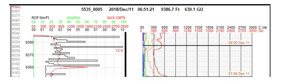
Although new data comes into the software's database every 6 seconds, the Main Screen is not automatically updated that frequently. This reduces the problem of the charts shifting while the user is trying to do something, such as make a depth correction. To manually refresh the charts with the most recently received data, the user may click on the Reset View button in the Chart Control Box (shown below):
