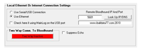
When Gas Chart software is being used at a location remote from the Bloodhound (running remotely), check the box next to "Use Ethernet" Instead of "Use Serial/USB Connection" and type in the 4-digit number of the Bloodhound and push the "Look UP IP/DNS" button, and the IP and Port will be displayed in the box below. Click on the red "Get Data From Bloodhound" to ensure connection (See Getting Started section for detail).
