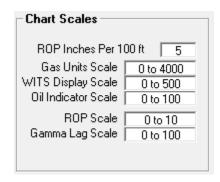
ROP Inches Per 100 ft 5 :- Changes the vertical scale of the ROP graph (bottom right of the Main Screen), and may be used to control the scale of printed output.
