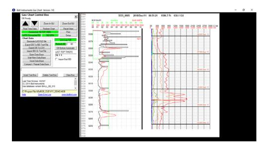
The Main Screen is a large chart divided in half by a thick black line at the center of the page. To the left and right of this line are two entirely different charts that are drawn in two different ways. The chart on the left is drawn by depth and will advance only when depth is being recorded. The chart on the right is drawn by time and will advance whether depth is advancing or not.
