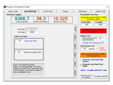
First, select the type of lag you are using by selecting either, Generate Lag using Pump Strokes or Generate Lag Using Time / Depth in the bottom-right corner of this page (See NOTE).
