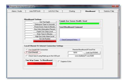
In the Edit box to the right of the Use Ethernet radio option you just selected, you will ONLY be concerned with the smaller Edit box to the Left of the Look Up IP/DNS button. Remove the unit number that is in that box and type in the Unit number of the Bloodhound you are using. Where XXXX is in the picture below is where you will type in your BH Unit number:
