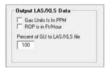
Gas Units Is In PPM Checking this box will generate the Total Gas column in your LAS/XLS file in Parts Per Million (PPM) rather than the default which is Gas Units, or the actual number displayed on the Bloodhound's LCD as Total Gas. PPM is one-thousand times the value of Gas Units.
