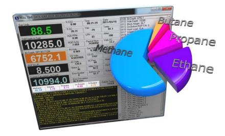
Using Gas Chart and the Bloodhound, the Bloodhound can capture, measure, and break apart C1 through NC5.
