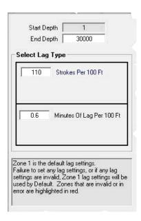
The setting will be saved upon closing the Setup window. Information can often be obtained from the Mud Engineer or Mud Report. For example, for a 7 7/8-inch diameter hole containing 4  $\frac{1}{2}$ -inch drill pipe, the annular volume of 1,000 feet of hole is about 41 barrels (bbls). For a pump with a capacity of 0.0725 bbls per stroke, it would take about 56 strokes to circulate 100 feet of hole. For a hole 5,000 feet deep, it would take about 2,800 strokes (5 x 560) to achieve bottoms-up.
