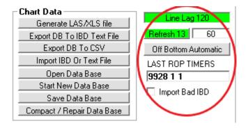
Line Lag is the time set on the Auto ROP/LAG tab, in the box below Surface/Line Lag.
