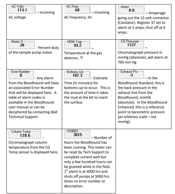
NOTE: Whenever more than one alarm condition is currently being met, the Error Description on this page will show "UNKNOWN". In those cases, the multiple Error Numbers will be displayed in the "Error Number" field on this page, separated by commas.
