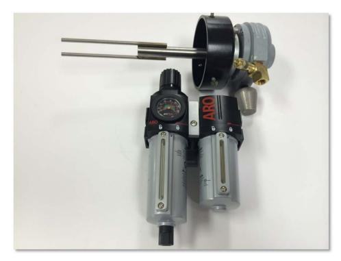
The Water trap has a built in water dump so that if water does collect in the line and trap, it automatically dumped when the float inside level reaches about an inch. Also, the regulator portion will the keep pressure nominal while the post oiler can maintain a mist of oil to the air motor beater assembly.
