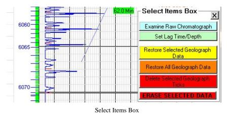
Examine Raw Chromatograph This button allows the user to see a close-up view of the selected chromatograph output. Left clicking and holding on the chromatogram will allow the user to adjust the trace up and down on the display window. If the trace is too large or too small, the user can adjust the overall visual size in the Program and Equipment Setup Screen, under the Chromatograph Tab. When the user is satisfied with the display, a print can be made of the chromatogram.
