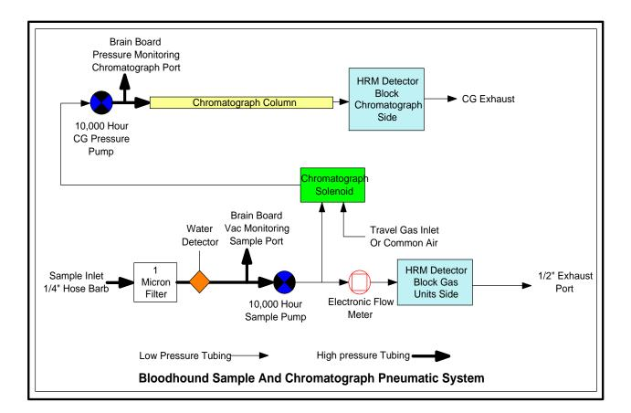
**NOTE:** The 1/2" exhaust must have a MINIMUM 1/2" exhaust tubing run from the Bloodhound to the external of the Logging Trailer or other housing.
