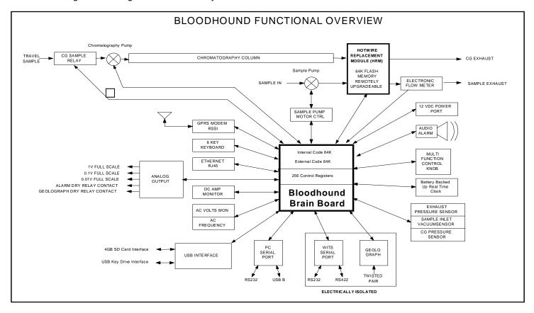
The Bloodhound is composed of an infrared detector, a proprietary chromatograph system, medical grade 10,000 hour brushless vacuum pumps, an aircraft grade flow meter, an uninterruptible power system, DC power input/output port, WITS (Wellsite Information Transfer Specification) communication, Ethernet connectivity, a wireless 3G data modem and the proprietary digital signal processing system Brain Board and housed in a rugged plastic Pelican case.
