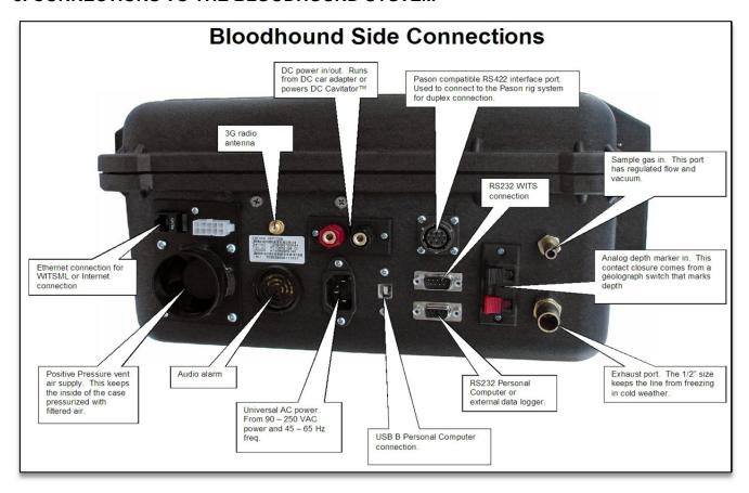
All outside connections are made to the external surfaces of the case to allow for the case to be closed when in operation.
