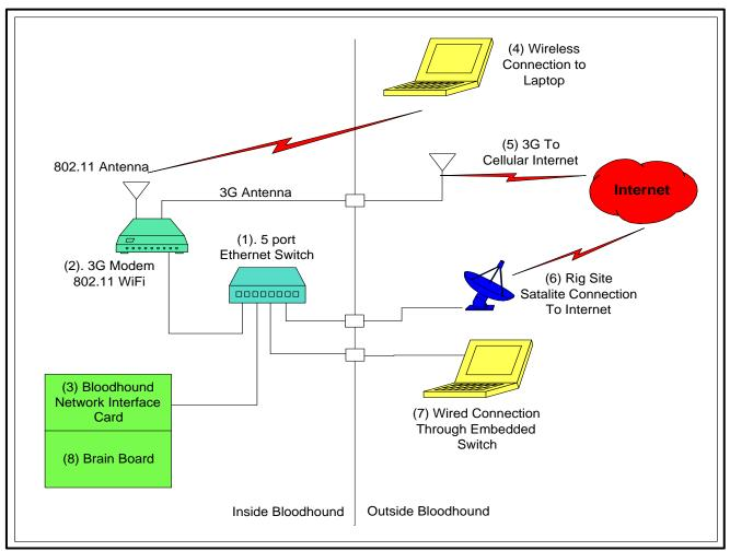
The connectivity of the Enhanced Bloodhound is expanded with the use of a 5 port Ethernet Switch, and an internal intelligent 3G modem.
